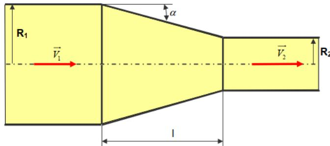
We want to accelerate the circulation of an ideal fluid in a pipe such that its velocity is multiplied by 4. To do this, the pipe has a converging section characterized by the angle  $\alpha$  (see the diagram above).
